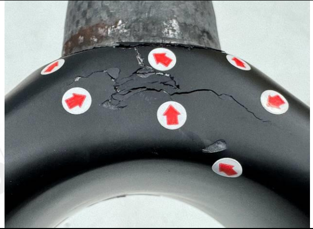
Photo "L" Appearance of sample after testing
